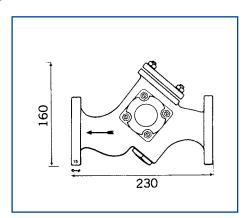
: flanged DIN DN20-PN40 **End connections**
